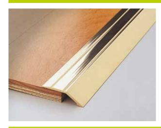
The LEVELTEC RP edge profiles can be used as trimming or to join floor types of different thicknesses. This profile section hides tile and carpet edge imperfections. LEVELTEC RP profiles have a sectional height ranging from 4.5 to 12.5mm and can compensate for elevation differences of 3 to 14mm. This product is equipped with heavy-duty adhesive, ready for installation.
